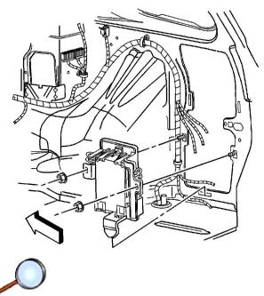
3. Install the module onto the vehicle.
