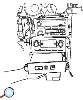
3. Align the communication interface module with the center stack I/P substraight and tighten the mounting screws.
