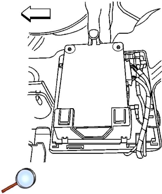
3. Remove the module from the upper bracket by releasing the retaining tab.
