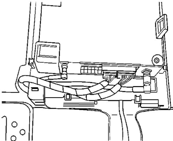
4. Remove the electrical connectors from the VCIM.
